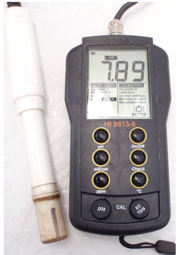
Figure 3. Select a combination pH and EC meter that is value priced, easy to calibrate, and reports EC in mS/cm.
